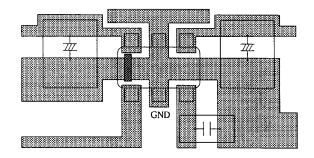
Make a large copper pattern as much as possible to have better heat dissipation. (pin 5 is heatsink)
