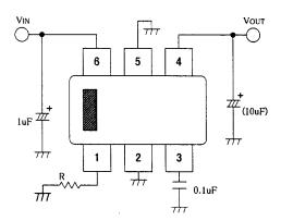
Connect control terminal to GND. R is good for quiescent current but bad for operation starting voltage (R:0  $\Omega \sim 300 \text{k} \Omega$ )
