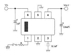
Noise pass pin is high impedance, so be careful to external noise if Cp is not used.
