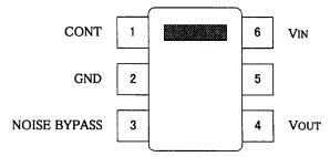
pin #5 to be grounded for heat dissipation
