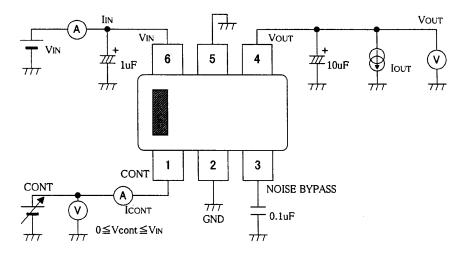
Pin #5 to be grounded for heat dissipation Tantalum capacitor to be used
